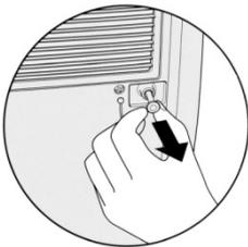
Remove the permanent drainage seal from the rear of the unit. To prevent this being mislaid this is attached to the rear of the panel of your dryer.
