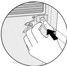
Ensure that the tube is securely attached to the drainage outlet and route the pipe ensuring that:
